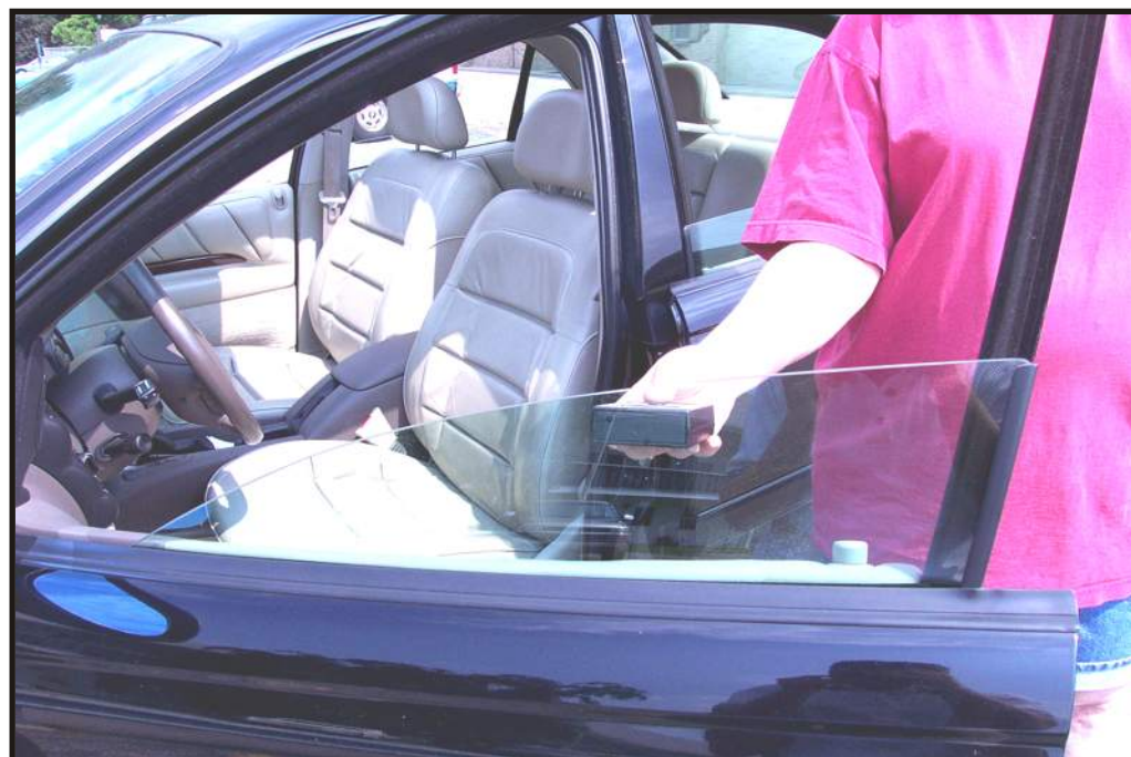
STEP 5: Meter measuring UV Transmission through car window.
